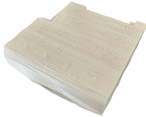
Figure 7: Failed 3D print of one-sixth of the full-sized board. Due to time and equipment constraints, structural integrity was impossible to achieve within this print. Pictured here is the distorted and flimsy product of 3D printing, resulting in our disbelief in 3D printing as a viable method of producing the full-scale radiological positioning board.
