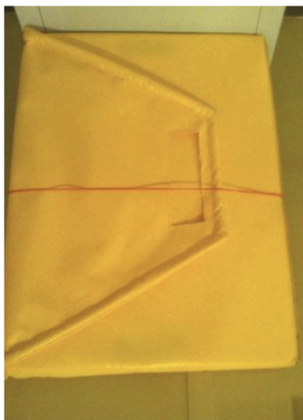
Figure 2: Current Design with Jingle Bells. Shown here is a design that attempted to prevent technologists from forgetting the board under a patient. Once the board is placed, these bells would be wrapped around the placer with string until its removal.
