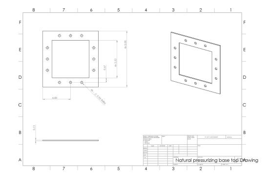
SolidWorks drawing of naturally pressurized base design with dimensions (view 1)
