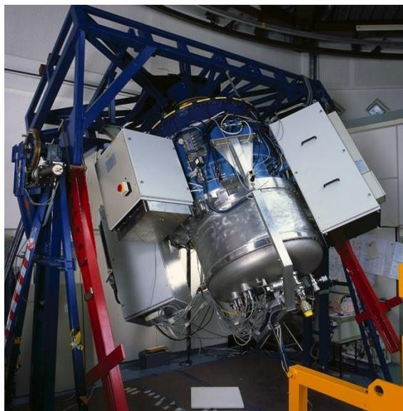
*Figure 3 SINFONI—a near-infrared integral field spectrograph—at the integration lab at the ESO Headquarters in Garching in 2004. Image credit: ESO (2004), <https://www.eso.org/public/belgium-fr/images/sinfoni-int-lab-hq2-03-04/>*
