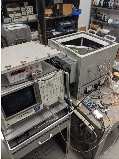
(a) Calibration test setup with HP 8753D VNA
