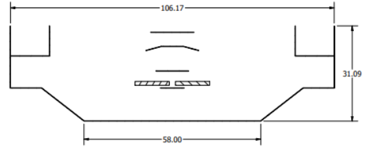
Figure 4.4: (Left) GBT310 Feed in the Field. (Top) Section View of GBT310 Feed
