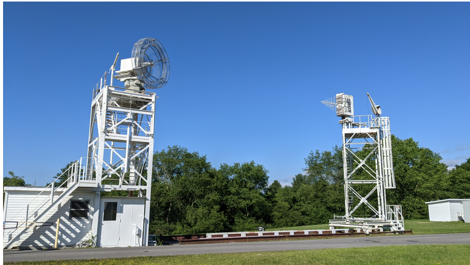
Figure 4.6: GBT 310 MHz feed at the Green Bank Observatory outdoor antenna test range. (July 2021)
