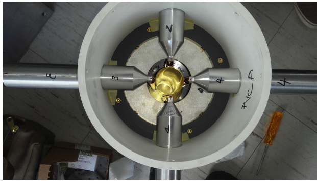
(a) Internal view of the GBT310 dipole assembly
