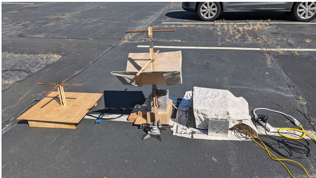
Figure 4.41: GBT310 receiver driftscan measurements with and without the balun assembly using a pair of janky homebuilt antennas with balanced-outputs (a corner reflector dipole and a cross-dipole). NRAO CDL parking lot, Oct 2, 2023
