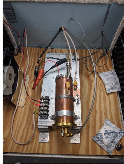
(b) Closeup of PAPER balun in Temperature Controlled Box.
