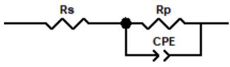
Figure 2.13. Circuit model used to fit the CPE parameters  $Q$  and  $\alpha$  and their evolution with time.
