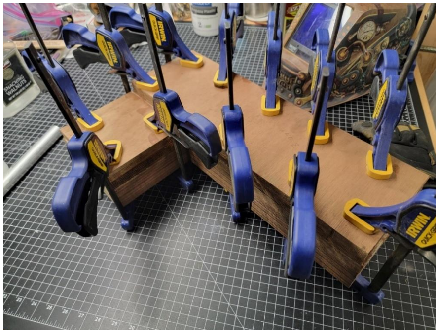
Fig. 3.3.4. Upper Playfield Plywood Stock Glued
