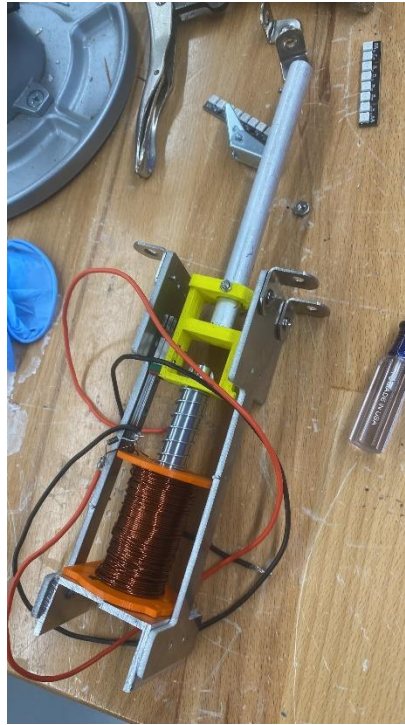
Fig. 2.3.6. Second iteration of pop bumper (pre-mounting)
