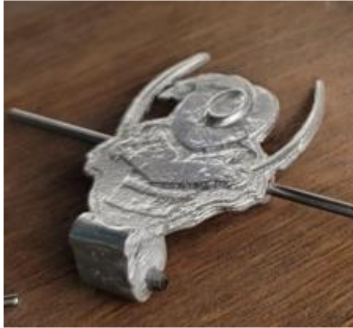
Fig. 2.8.5. Final sand-casted version of the Cavman spinner with tungsten weight
