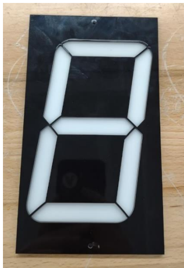
Fig. 2.10.1. Single acrylic digit prototype
