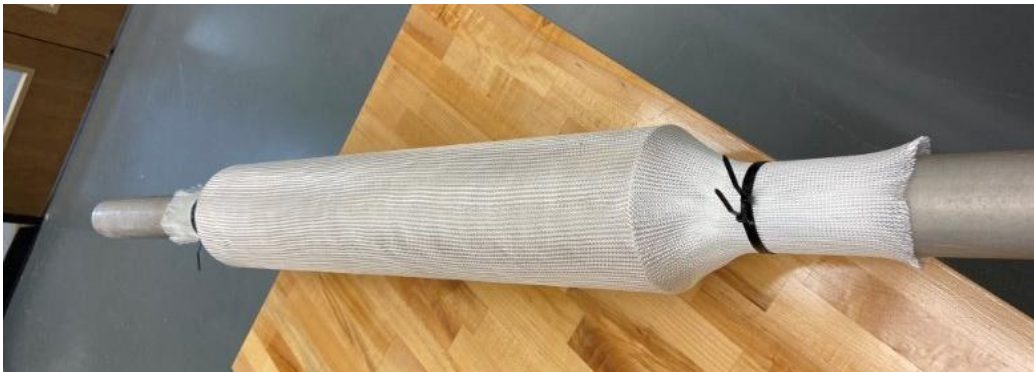
Figure 63. Fiberglass sleeve fixed over phenolic tubing.
