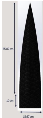
Figure 3. Final ogive nosecone design and dimensions.
