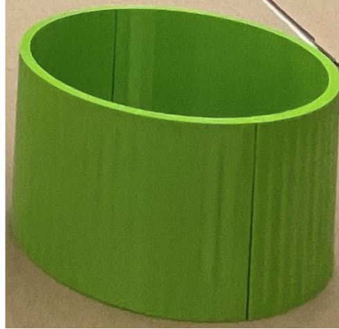
Figure 55. Extended nosecone mold (Height 10 cm)
