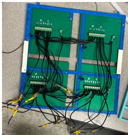
Figure 7 Button PCBs with Rows and Columns Connected
