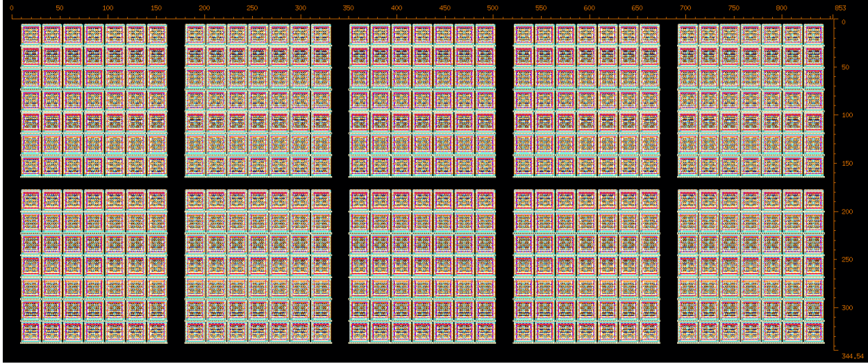
Figure 3.1: The estimated total capacitor can be placed in 80% of 0.4 mm 2 , 1.149nF placed in 853um x 344.54um
