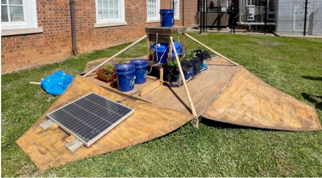
*Figure 6. Floating platform, unfolded.*
