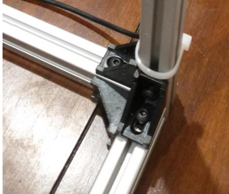
Figure 7: Rail System Joints
