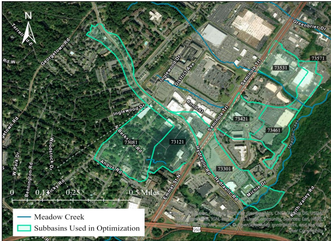
Figure 13. Detailed view of subbasins used in the PySWMM optimization.
