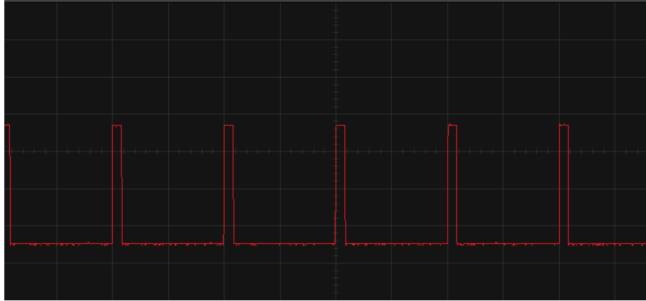
Figure 42 Servo Signal without Motor Running
