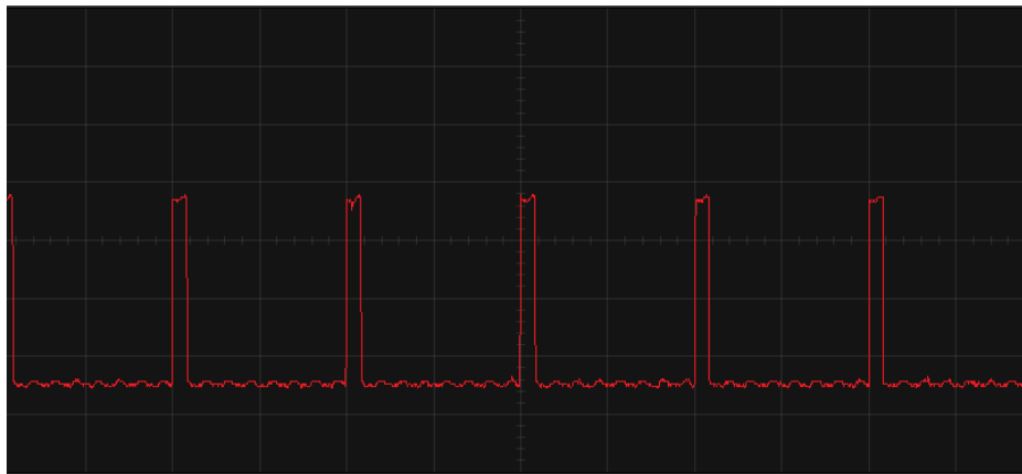
Figure 43 Servo Signal with Motor Running
