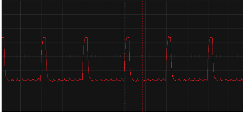
Figure 44 Servo Signal with Lowpass Filter
