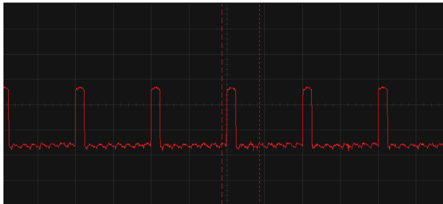
Figure 45 Servo Signal with Voltage Divider
