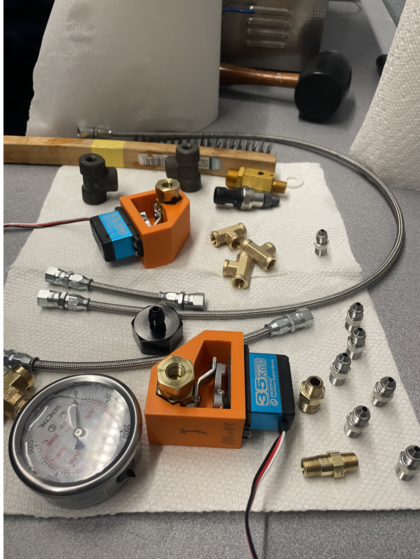
Figure 14: Assorted oxidizer plumbing components, including analog pressure gauge and servo-actuated ball valves, after cleaning.
