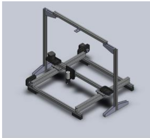
Figure 2: 3D CAD of the gantry
