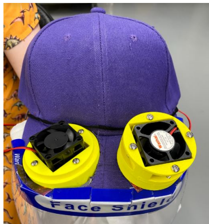
Figure 7: The second prototype with the two kinds of fan casings attached.
