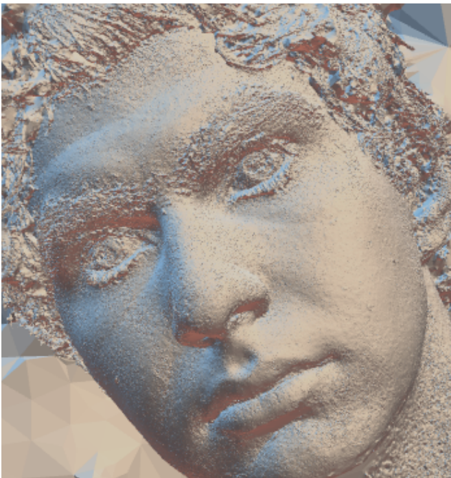
Supplemental Fig. 2. 3D mesh model generated using an iPhone 12 1x camera lens
