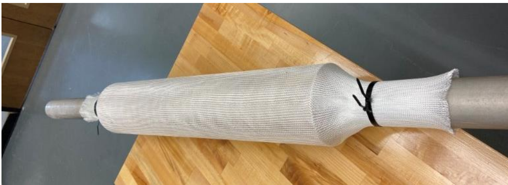
Figure 63. Fiberglass sleeve fixed over phenolic tubing.
