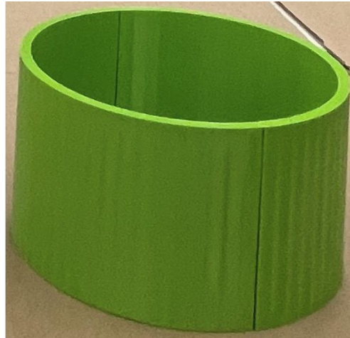
Figure 55. Extended nosecone mold (Height 10 cm)
