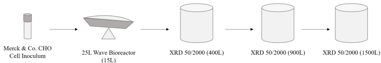
Figure 4.1.2. Fed-batch inoculum train equipment and working volumes from 4.5 mL vial to 1500 L perfusion reactor.
