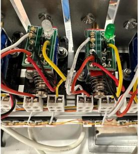
Figure 9 Example Mount for the Solenoids
