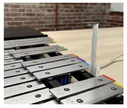
Figure 11 Microphone Connected to the Xylophone
