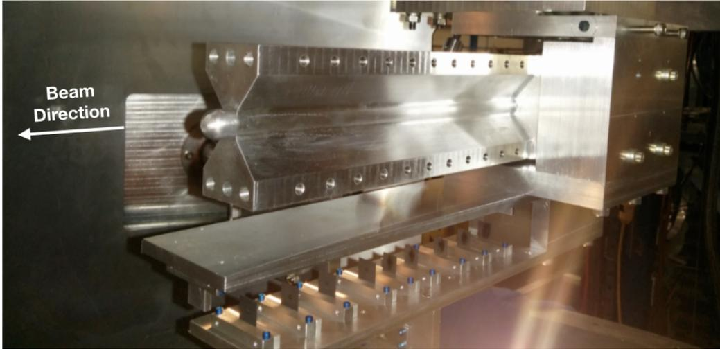
Figure 30: Photograph of the Hall A target ladder used in E12-14-012, showing the argon gas cell (top), the aluminum dummy target (middle), and the carbon optics target (bottom)[10]. The beam (arrow) enters from the far right, and exits the target tube at the left of the photograph.
