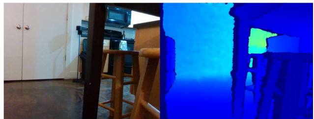
Fig. 3: Images provided by the RealSense D435 camera showing both an RGB image (left) and the depth view of the same scene generated by its
