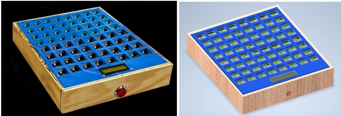
Figure 5 Final Mechanical Housing (left). CAD Model (right)
