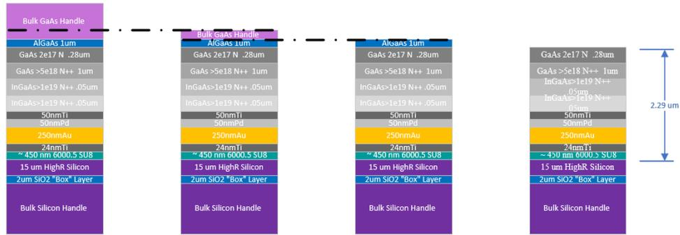
Figure 33 – Cartoon illustrating the GaAs handle removal process
