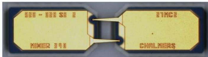
Figure 5 – Photograph of Chalmers Antiparrel Schottky Diodes[30]
