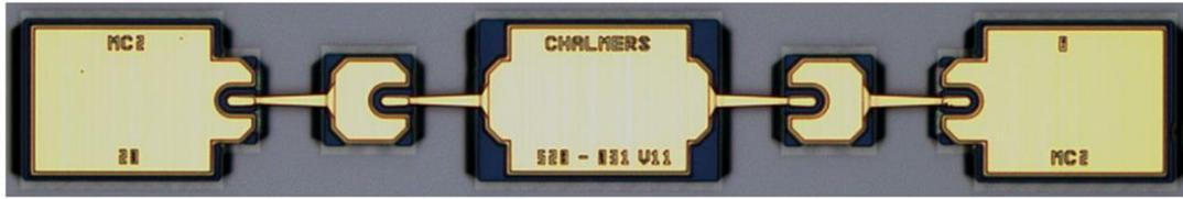
Figure 6– Photograph of Chalmers AntiSeries Schottky Diodes [30]
