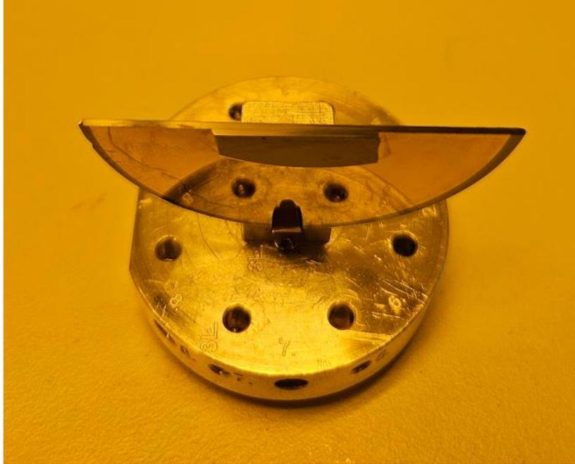
Figure 56 – The diced wafer mounted for SEM imaging.
