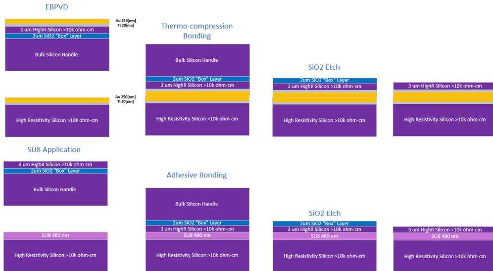
Figure 58- Abbreviated fabrication process for this SU8 vs. metal-to-metal experiment.
