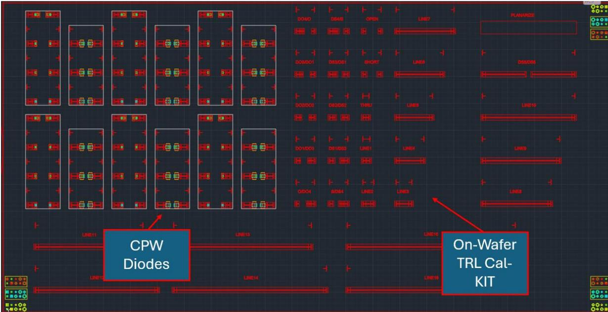
Figure 68 – Experiment region with CPW diodes and CPW TRL Cal kit
