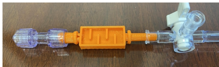
Figure 2. Dr. Thiele's original prototype for the disposable cartridge through which the fluid will flow.
