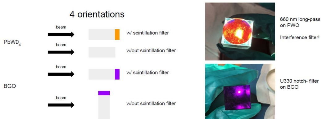
Figure 1.18: 4 Primary configurations were tested. The first two observed PbWO 4 placed parallel to the beamline either with or without the 660 nm interference filter. Other configurations used BGO crystal with an absorption filter in both cases, either along the beamline or oriented perpendicular to the beam. The PbWO 4 is the focus of this analysis. Credit: Grace Cummings.
