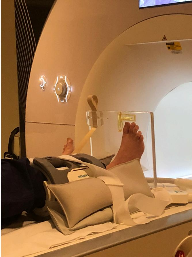
Figure 9: First stage prototype ergometer
