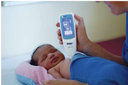
Figure 1: Portable Jaundice Meter-Bilirubinometer. Source: Courtesy of M/s Dragerwerk AG & Co. KGaA.
