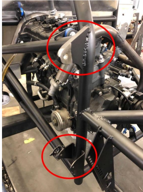
Figure 37: Welded mounting tabs for the rocker and linear actuator
