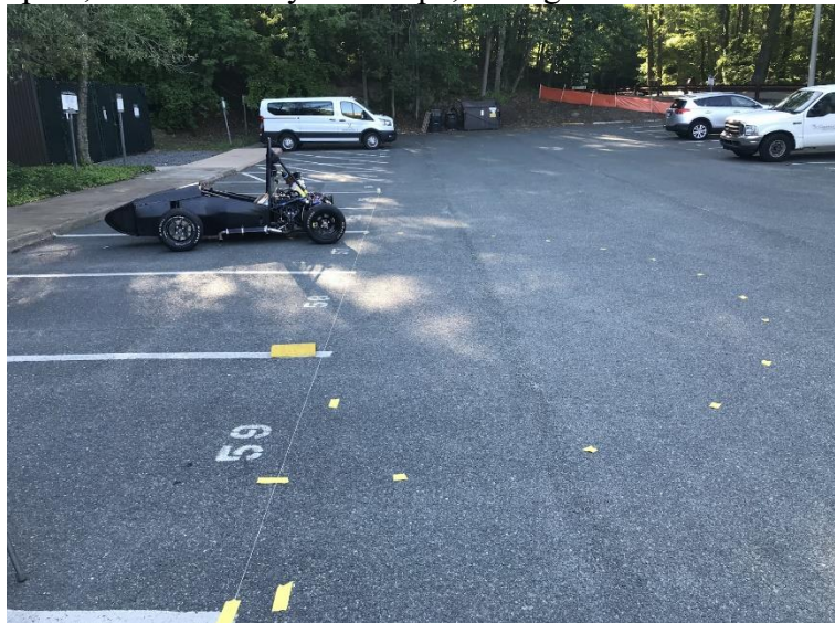
Figure 42: Turning radius test without rear wheel steering. (3.38 m turning radius).
