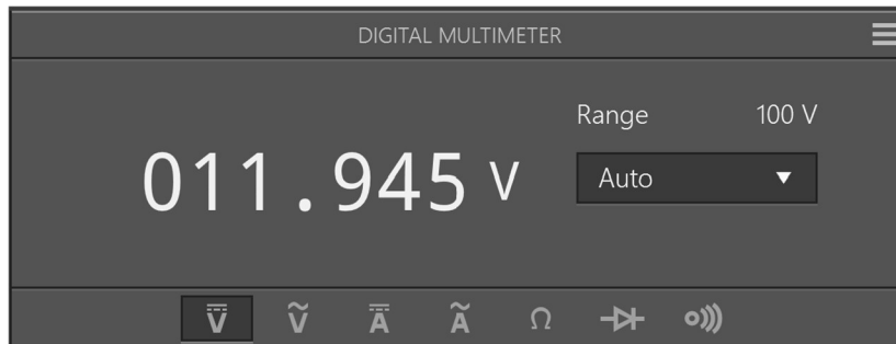
Figure 33 Voltage into Positive Terminal of Electric Strike
