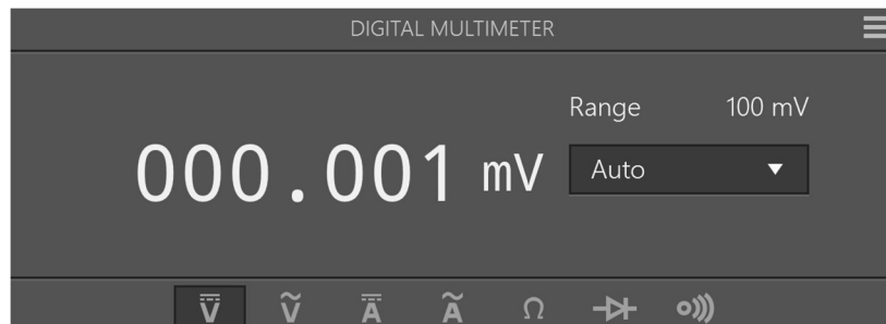
Figure 49 Voltage across Electric Strike when Unlocked without Wall-Plug Power Supply
