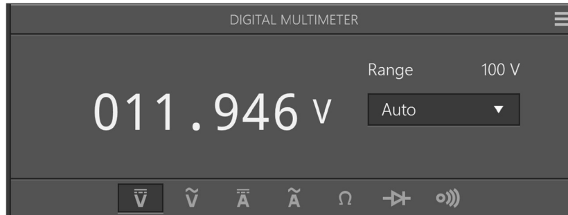
Figure 48 Voltage into Negative Terminal of Electric Strike when Unlocked without Wall-Plug Power Supply
