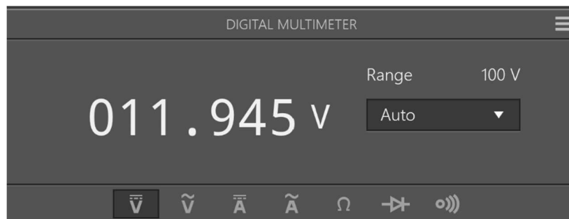
Figure 39 Voltage out of 12V Linear Regulator without Rechargeable Batteries
