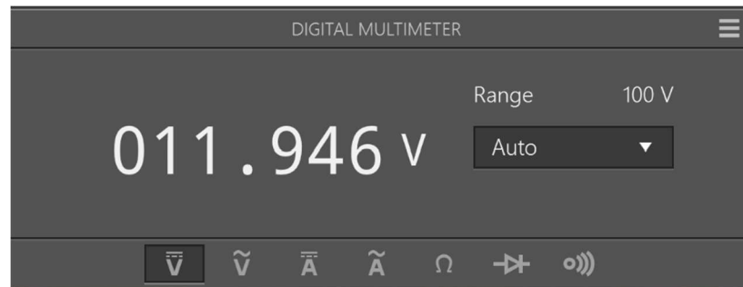
Figure 34 Voltage into Negative Terminal of Electric Strike when Unlocked
