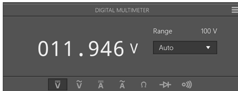
Figure 31 Voltage out of 12V Linear Regulator
