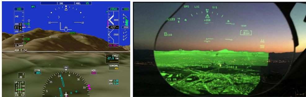
Figure 12.7: Examples of SVS (left) and EFVS (right) Displays
