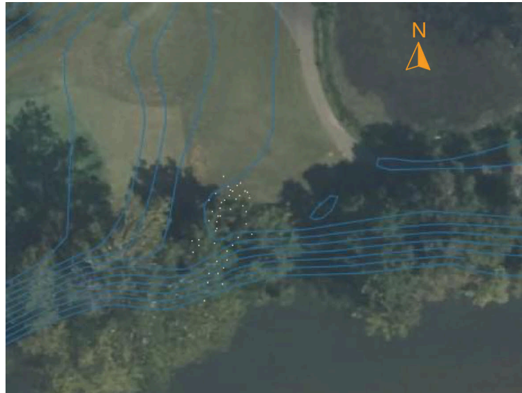
Figure 11: Headcut Survey Data with existing contours
