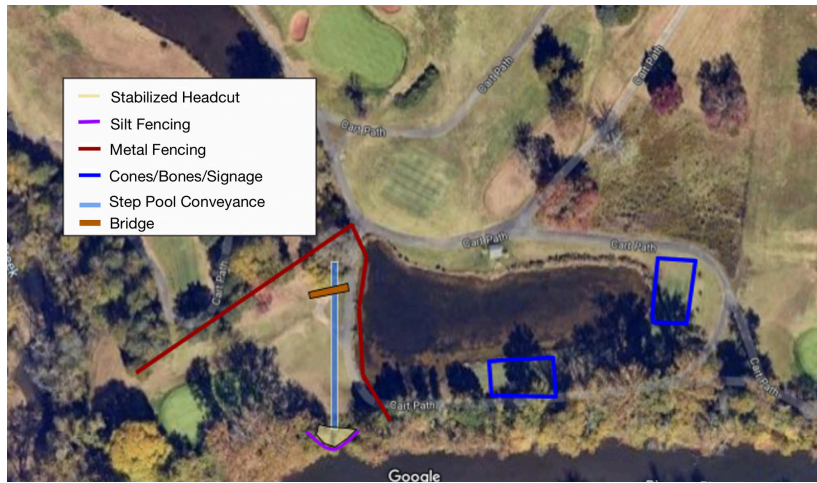
Figure 13: Construction Feasibility Mockup – Spatial Plan
