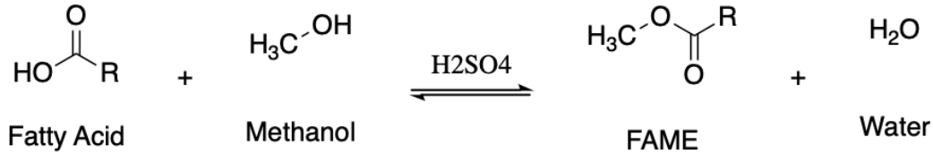
Figure 3.7-01: Esterification of free fatty acids into FAME.
