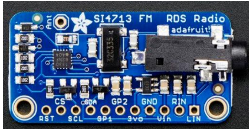
Figure 11: Adafruit Breakout Board for Si4713
