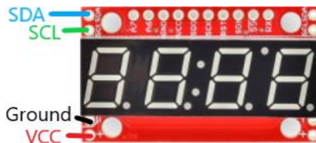
Figure 6: I2C lines for LED Display
