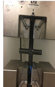
Figure 22: Tensile test setup
