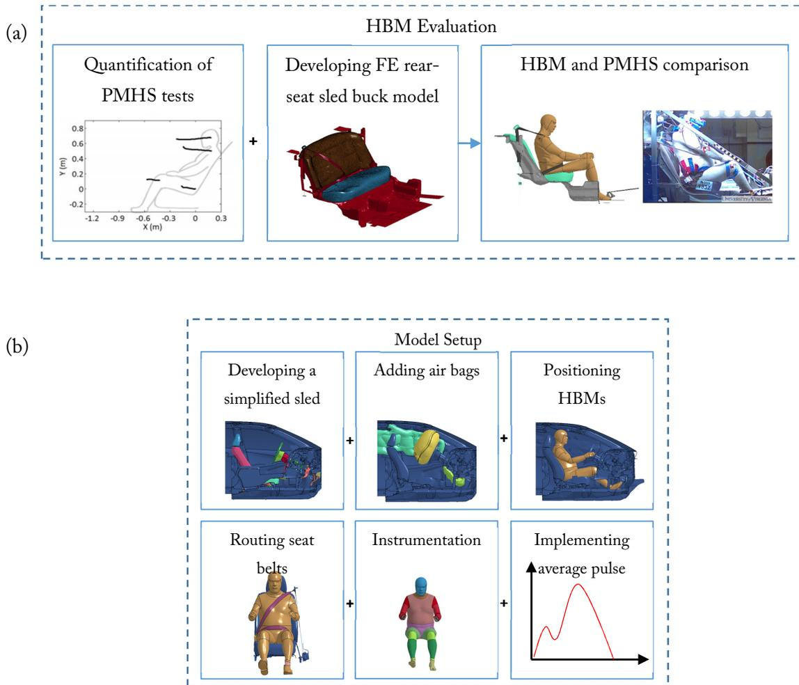
Figure 2: HBM evaluation (top) and model setup (bottom)
