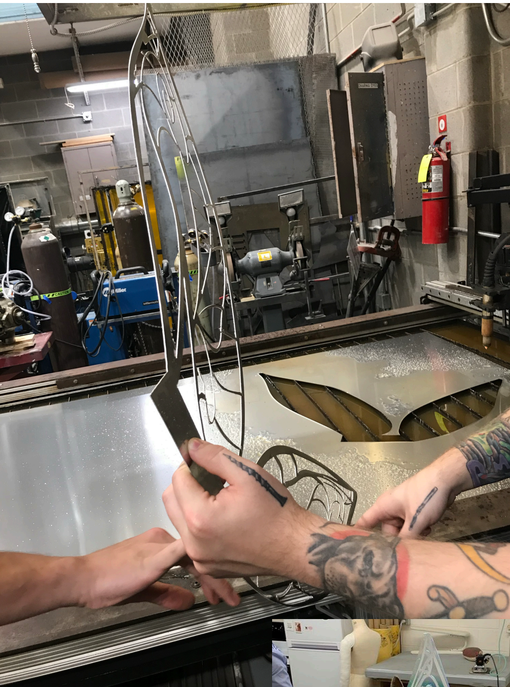
Above: Technical Director Chris Rybitski and MFA Technical Direction Graduate Student Jamie Nicholas Inspect the cut aluminum form
