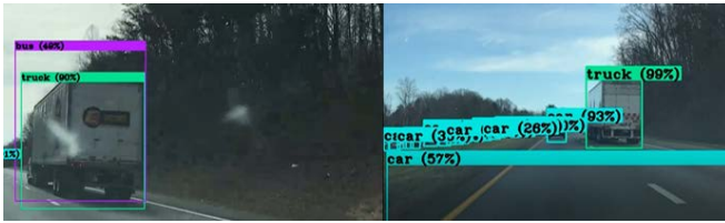
Fig. 15. Truck – False Positive and True Positive (YOLOv3)
