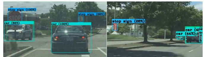
Fig. 12. Stop Sign - True Positive and False Positive (YOLOv3)
