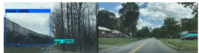
Fig. 14. Train vs. House - False Positive and True Negative (YOLOv3)
