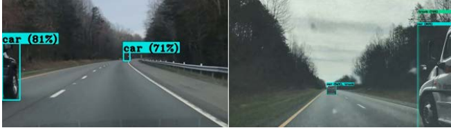
Fig. 16. Detect Objects that are Not Fully Captured (YOLOv3)
