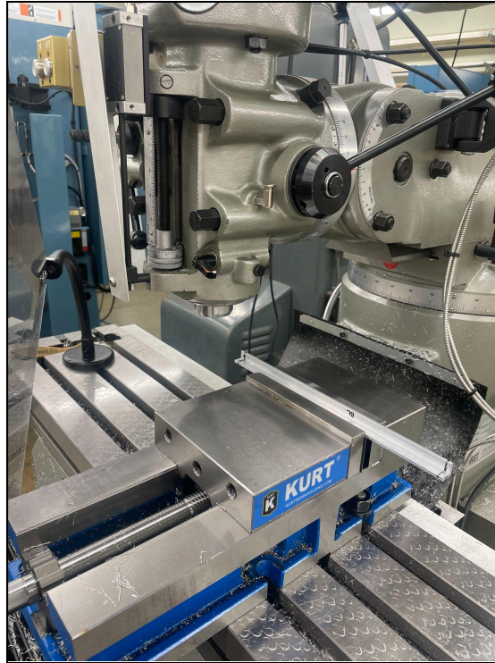
Figure 3H: Angle brackets in vertical milling machine
