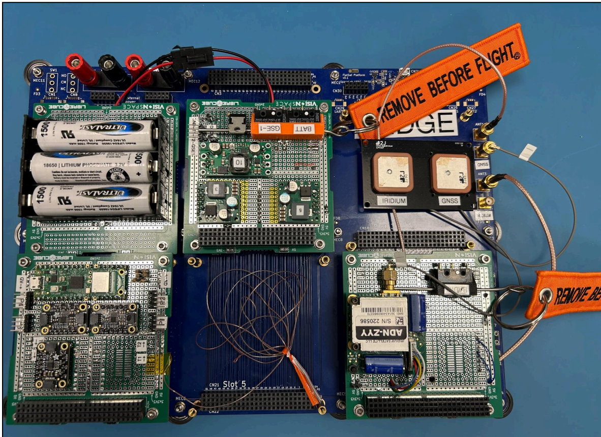
Figure 1J: Avionics Setup on Flatsat
