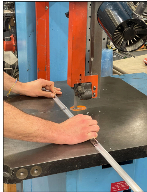
Figure 2H: Angle brackets cut with bandsaw
