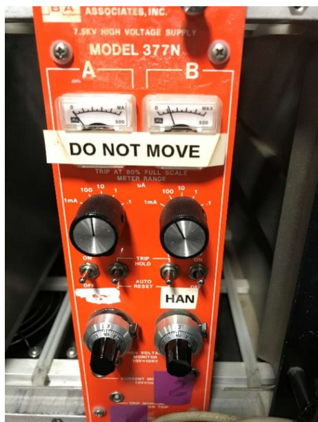
II Fig 4. 3 Wire chamber HV supply and HV distributor.
