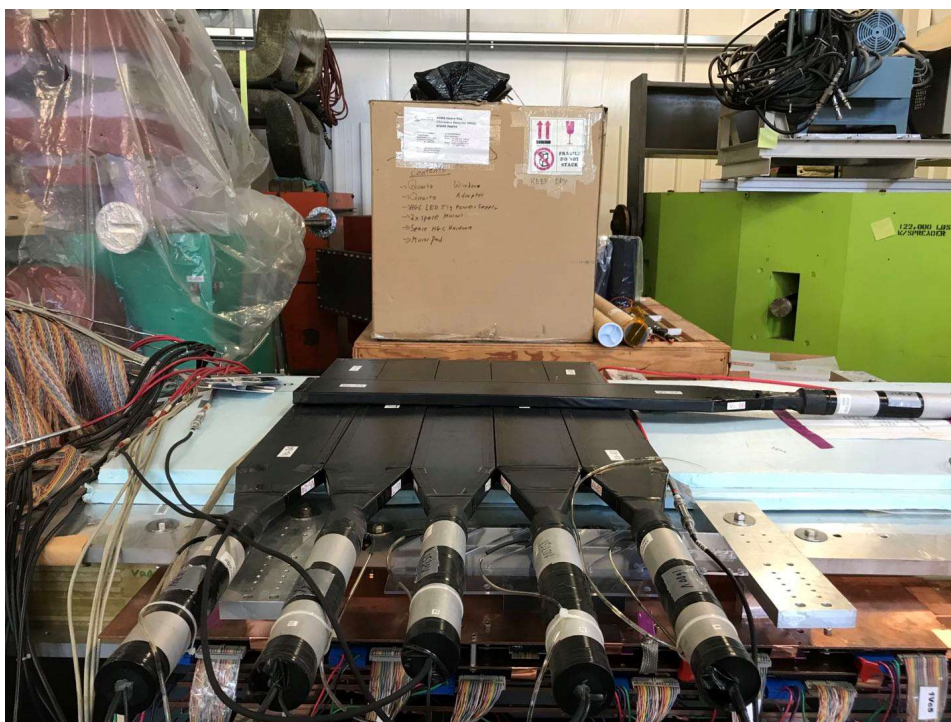
III Fig 5. 2 Upper chamber trigger and reference scintillators.
