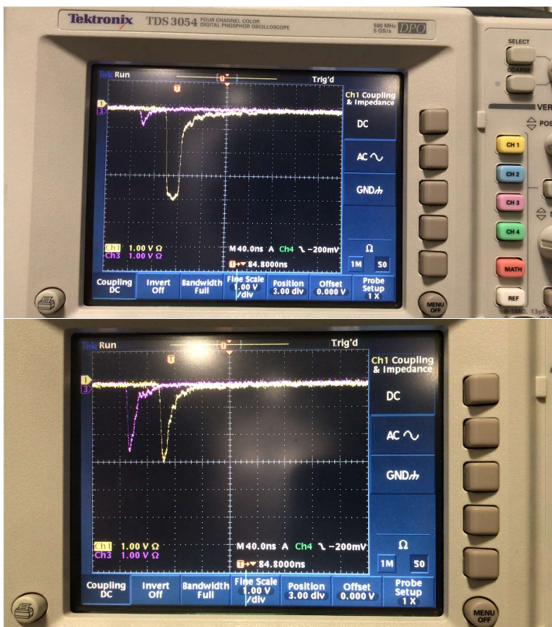
II Fig 5. 9 Pulse shape of two PMTs before and after gain match. Ordinate: pulse height in unit V , abscissa: time in unit 40 ns .
