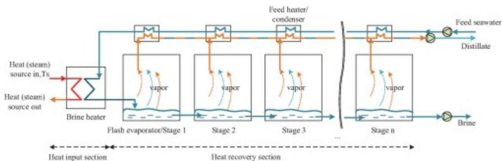
**Figure 3.4.1:** Diagram of Multi-Stage Flash Distillation Process (Rosen & Farsi, 2017)
