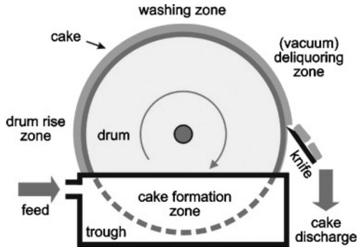
**Figure 3.4.6:** Rotary Drum Filter Diagram
