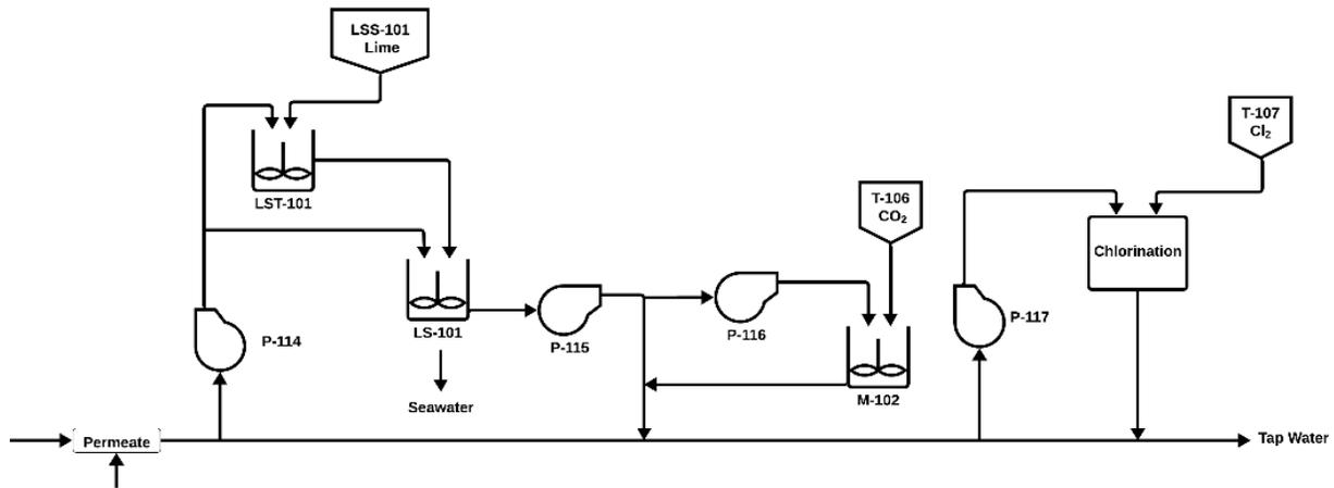
**Figure 4.3:** PFD for Permeate Post-Treatment
