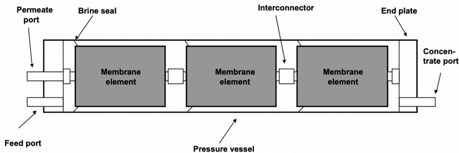
**Figure 3.2.3:** Pressure Vessel Depiction with RO Membrane Elements Inside
