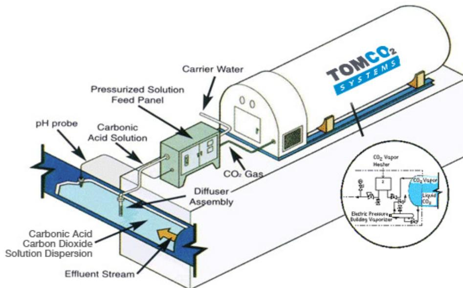
**Figure 3.3.2.** TOMCO<sub>2</sub> Systems' Pressurized Solution Feed System (TOMCO<sub>2</sub>, 2018)
