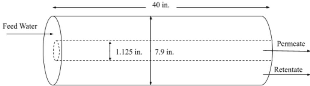
**Figure 3.2.2:** Diagram of RO Membrane Element Dimensions
