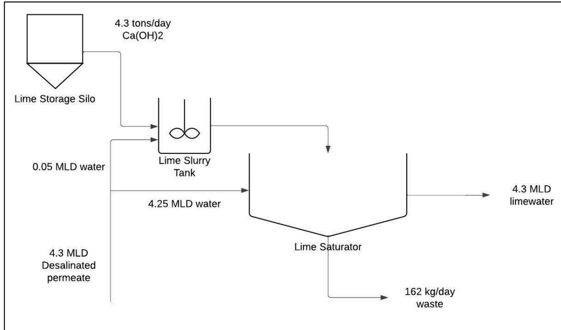
**Figure 3.3.1: PFD for Lime Addition**
