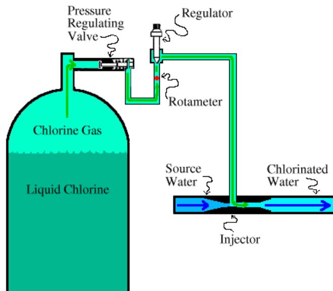
**Figure 3.3.3.** Vacuum Chlorination System (Chlorinator, 2024)
