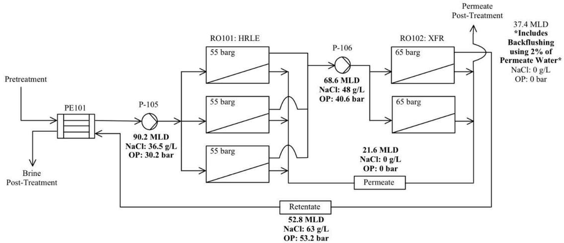
**Figure 3.2.1:** Reverse Osmosis Process Flow Diagram
