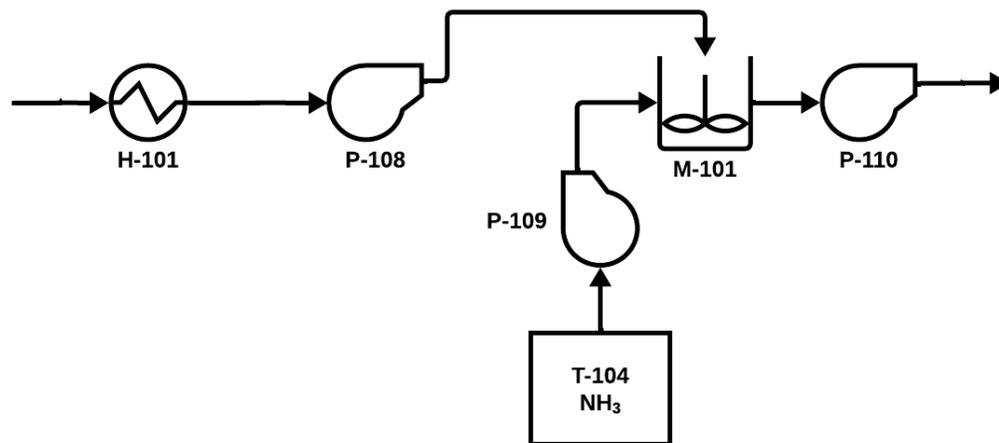
**Figure 3.4.4:** Diagram of Heat Exchanger PFD
