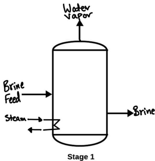
**Figure D:** Example of Stage 1 in Evaporation Unit
