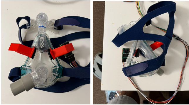
Figure 7. This is the front and back of the physical apparatus with the mounts seen in the front and the wired camera seen on the left side in the image from the back.
