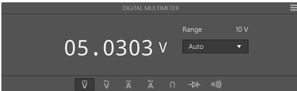
Figure 48: U2 Pin 8 Vcc Verification
