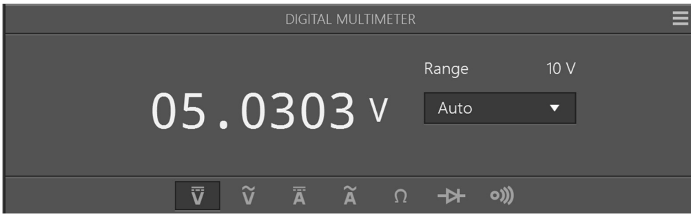
Figure 50: U3 Pin 8 Vcc Verification
