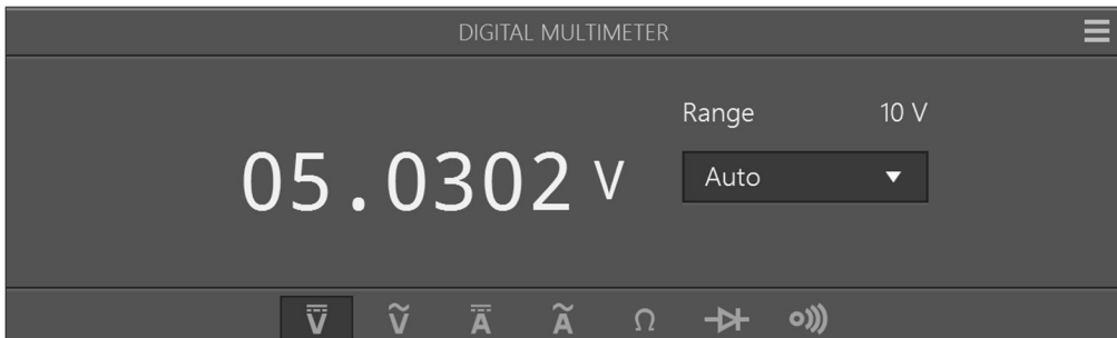
Figure 54: U10 Pin 8 Vcc Verification
