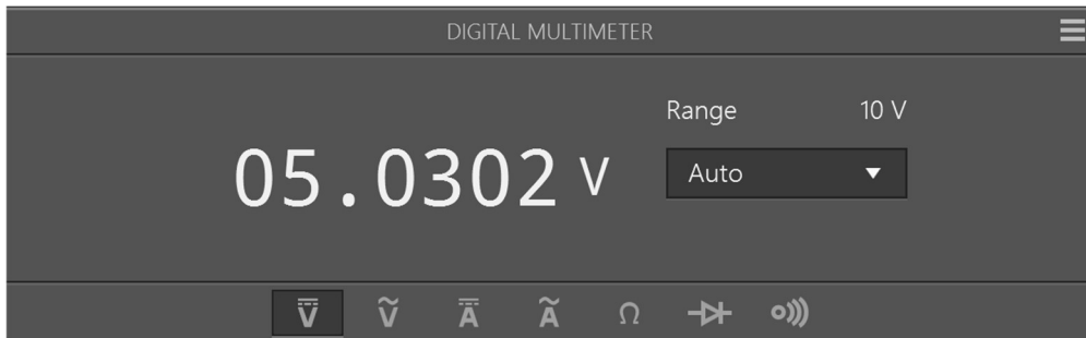
Figure 46: U7 Pin 7 Vcc Verification
