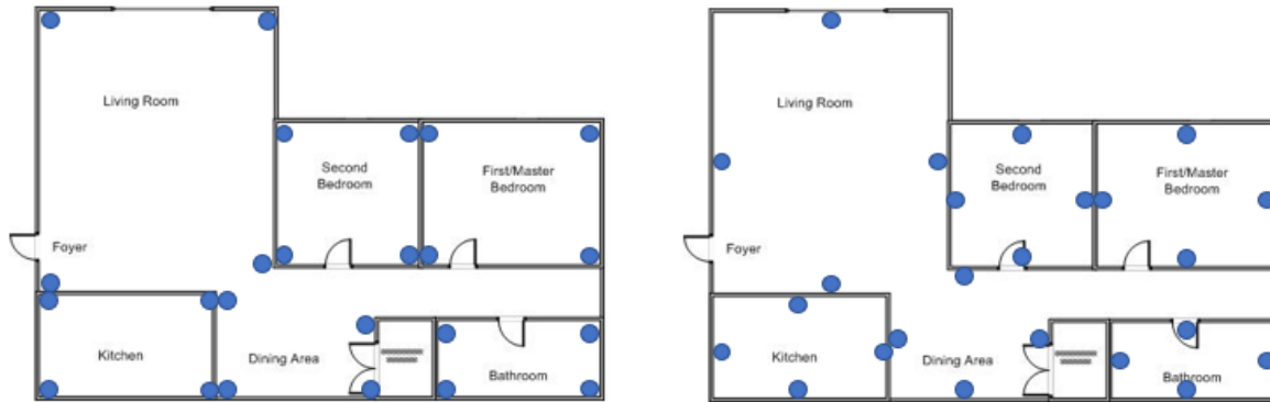
Figure 6. Displays an example deployment of all beacons positioned in the (1) Room Corners or (2) Center Walls.
