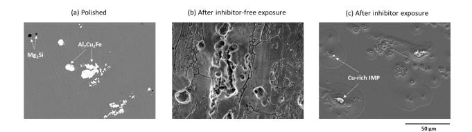
Figure 2.6. SEM images of AA7050-T7451 surface after (a) polishing, (b) 1 h OCP exposure followed by cathodic polarization in 0.6 M NaCl, and (c) 1 h OCP exposure followed by cathodic polarization in 0.6 M NaCl +  $10^{-2}$  M Na<sub>2</sub>CrO<sub>4</sub>, under quiescent conditions.
