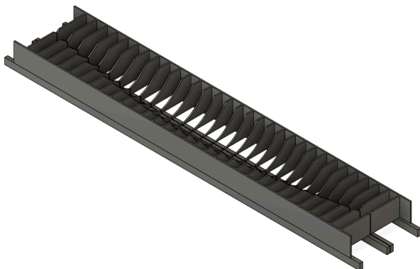
Figure 11. Detailed Design for Reusable Female Mold
