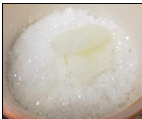
Figure 4.12: Synthesized 3-(4'-vinylbenzyl)-5,5-dimethylhydantoin or VBDMH monomers
