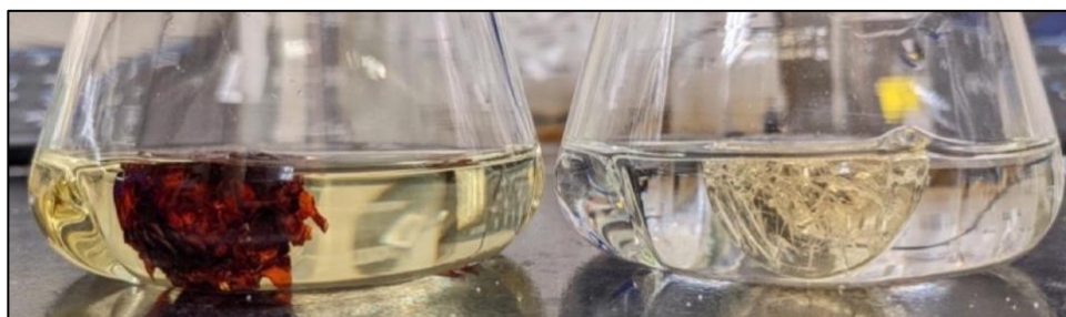
Figure 4.20: Iodide staining test for a chlorinated gel (left) and a non-chlorinated gel (right)
