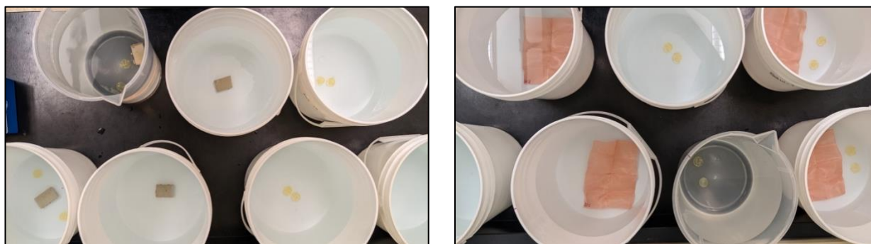
Figure 5.1: E. coli inactivation tests combining the chlorinated polymer gels with the MadiDrop+ or the copper screen, 8-h treatment in 5-L synthetic groundwater
