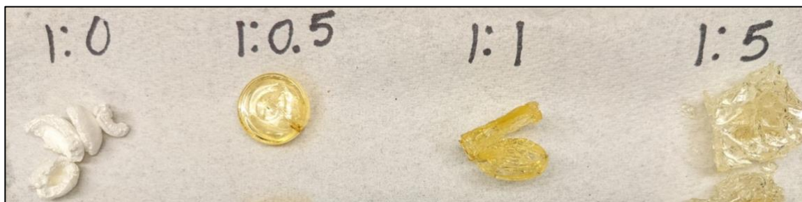
Figure 4.15: Polymer gels with varying VBDMH:PEGMA molar ratios (see formulations in Table 4.1)
