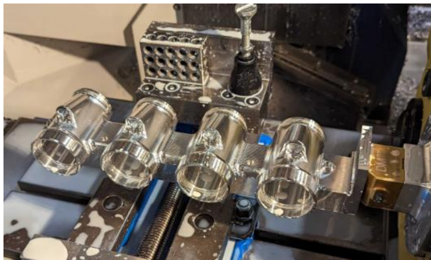
Figure 29: Semi-finished runners in 5 axis trunion.
