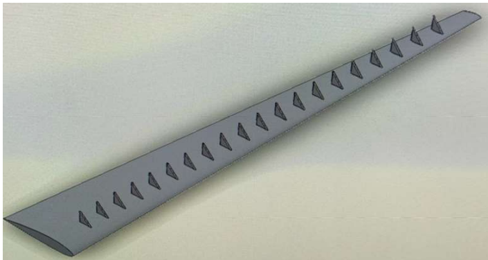
Figure 2. Thin nodes attached to leading edge (Jacobson, 2020)
