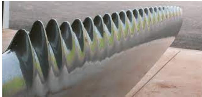
Figure 2: Tubercles on leading edge of wind turbine blade (Hamilton, 2008)
