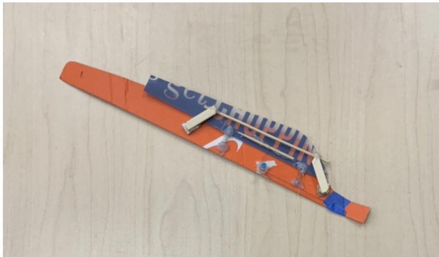
Figure 10: First Prototype of Spring-String Mechanism
